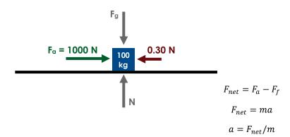
Level 2: A steel cube counterweight with a mass of 100kg is sitting on an asphalt road. The coefficient of friction between the weight and the road is given as 0.30. The road is at a  $25^{\circ}$  slope as shown below. If the counterweight is pushed on its side as shown with 1000 newtons, how fast would the counterweight accelerate in m/s<sup>2</sup>?
