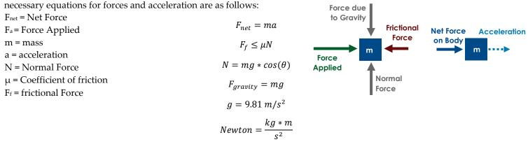
Newton's second law of motion states, "The force action on an object is equal to the mass of that object times its acceleration, F=ma." This law applies directly to free-body diagrams. Adding together forces applied will cancel out equal and opposite forces, revealing the net force applied. Using the net force with the equation F=ma will allow you to calculate an object's acceleration in that direction. An illustration of cancelling terms in a free-body diagram is shown above.
