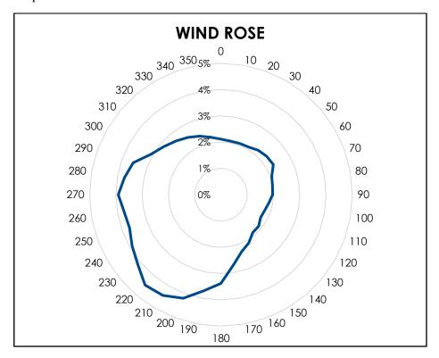
The percentage of wind from each direction is calculated by dividing the amount of wind (usually measured in hours per year or sample) by the total wind (total hours per year or sample).
