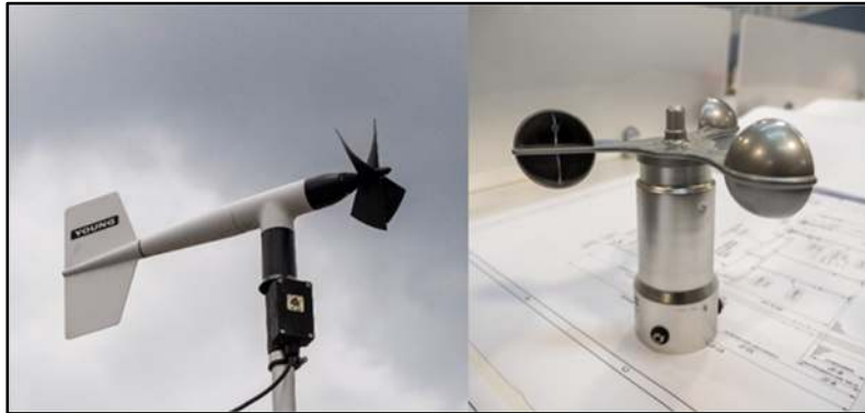
Figure 1: Vane Anemometer (left) and Cup Anemometer (right)
