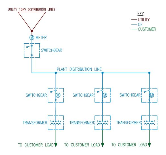
ONE-LINE DIAGRAM DEPICTING ONE ENERGY'S MANAGED HIGH VOLTAGE SERVICE AND HOW IT INTERCONNECTS WITH THE CUSTOMER'S FACILITY
