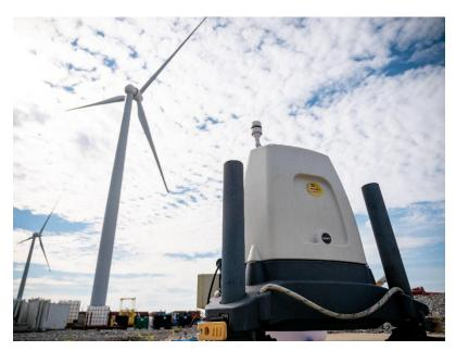
The LiDAR unit can measure wind speed at the same height as the turbine behind it, despite being over 76 meters shorter!
