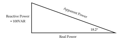
We also know that one of the angles must be 90°, because real power and reactive power are distinct from each other. Also, the interior angles of a triangle must add up to 180°. We have two of those measurements, 90° and 18.2°, so the third angle must be 71.8°.
