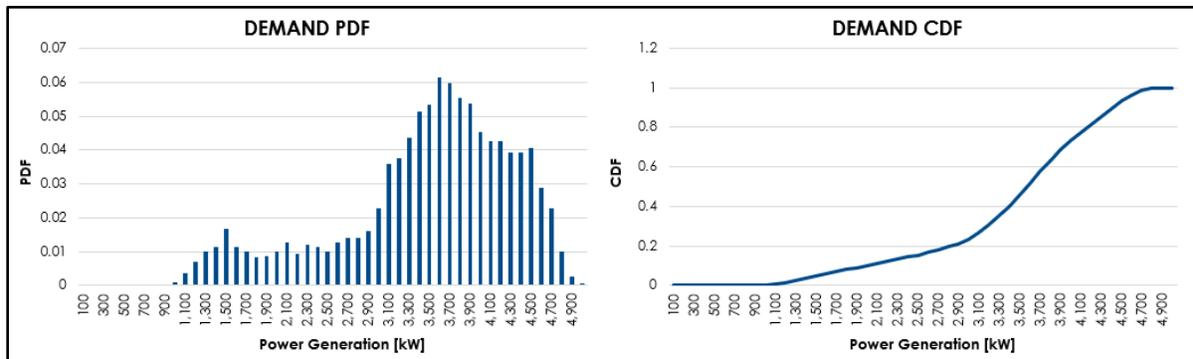
Figure 1: Load Distribution Example
